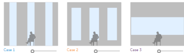
Figure 4. Three glazing scenarios with 40% window-to-wall ratio
